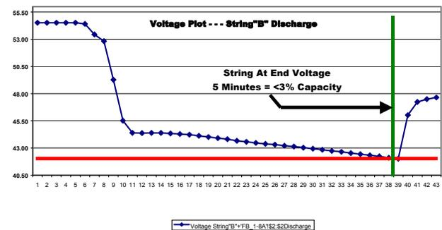
**Figure 3: 125 Ah = String Capacity Failure**
