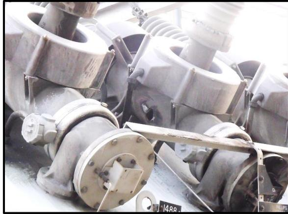
The center phase ruptured, all the SF<sub>6</sub> was released to atmosphere. The force of the blast shattered porcelain and damaged nearby equipment. This failure cost the utility over \$250,000. Disassembly of the other two poles revealed standing water puddled at the base of the interrupter.
