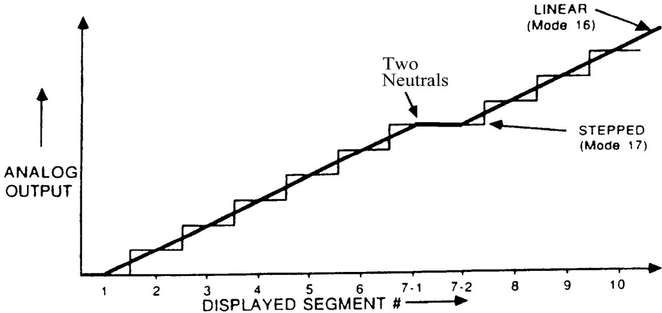
**Figure 2.3 Base 1 Uni-polar Mode Analog Output**
