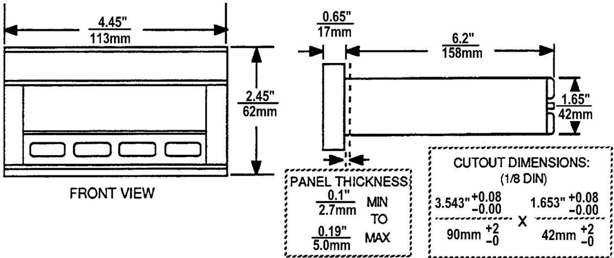
Figure 1.1 Mechanical Dimensions
