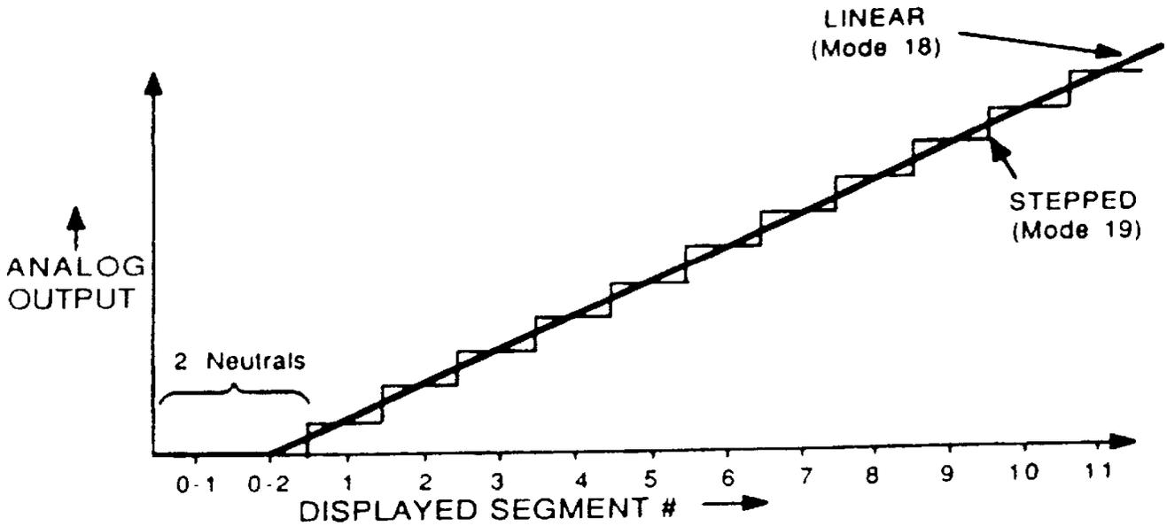
**Figure 2.4 Base 0 Uni-polar Mode Analog Output**
