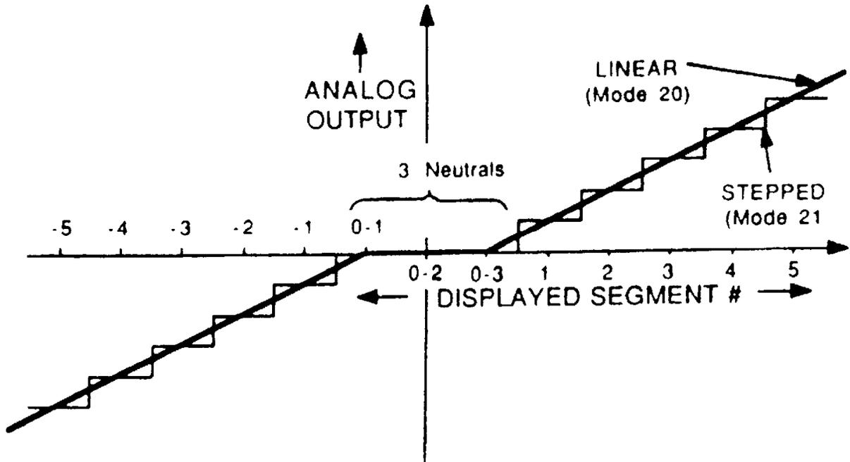
**Figure 2.5 Bi-polar Mode Analog Output**
